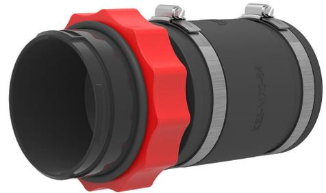
For use in wall insert and aluminium flange HSI90. For connecting smooth cable ducts. The seal is created with the sleeve method, with a rubber sleeve being clamped onto both the system cover and the duct with clamping straps.
