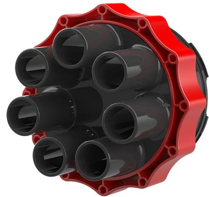
For use in wall insert and plastic flange HSI150. The cold shrink sleeves support a wide area of application. They are shrunk onto the cables by the system cover socket without tools. Empty system cover sockets can be sealed with blind plugs.
