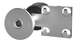
For installation flush with the formwork in waterproof concrete. Earthing connections can be made on the inside and outside with the thread on both sides in the conductor core. There is a tab with cross-clamp for making an earthing connection in the wall.
