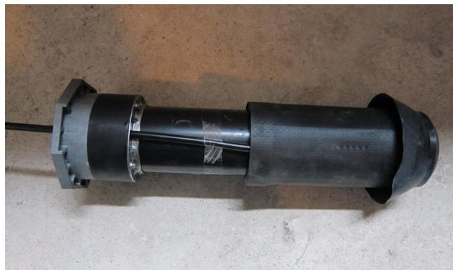
Adaptation of the building entry to the on-site conditions: cutting to length and adaptation to wall thickness. Sealing is achieved through injection of a 2-component resin via a filling hose.
