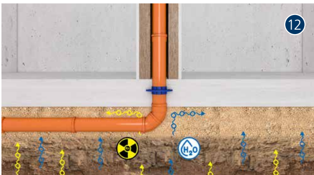
KGF110 set in concrete
