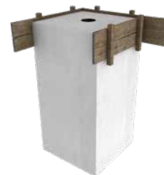
Foundation concreted on-site
