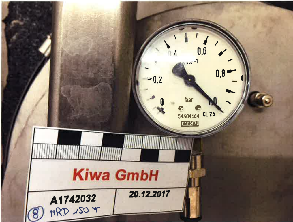
Figure A1. Water tightness test with \geq 1,0 bar water filled test cylinder (manometer at the beginning of testing on 20.12.2017).
