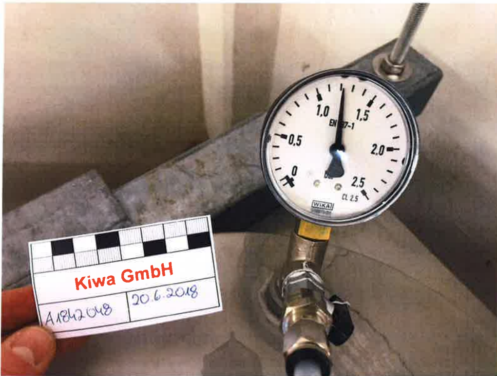
Figure A1. Water tightness test with \geq 1,0 bar water filled test cylinder (manometer at the beginning of testing on 20.06.2018).
