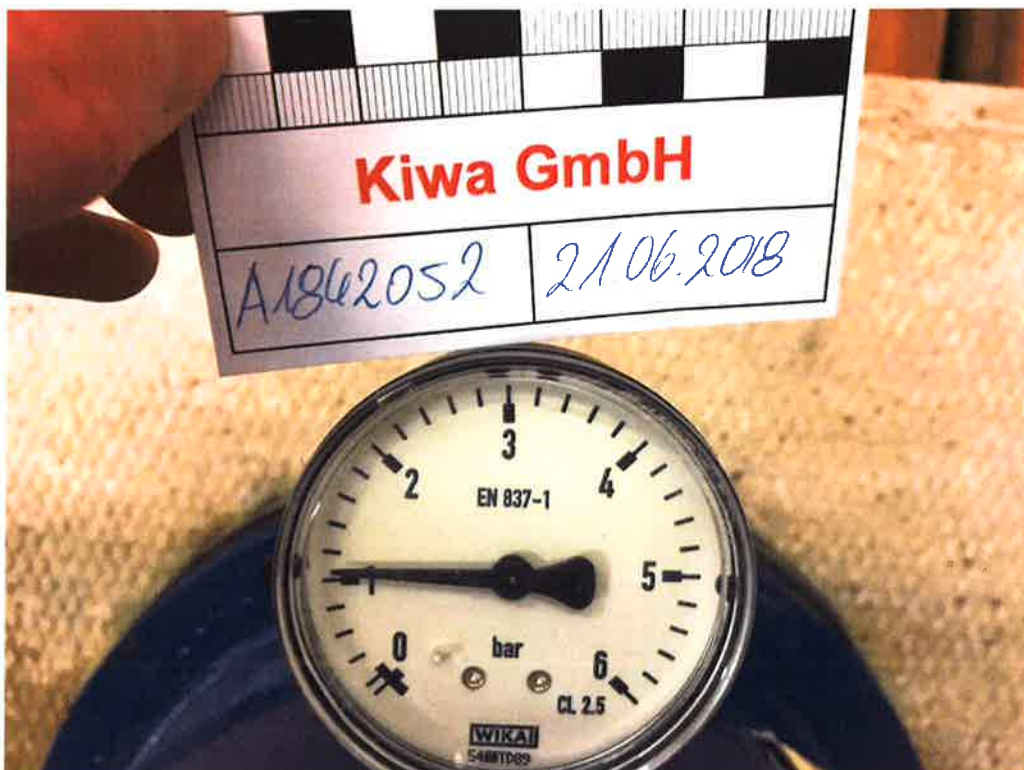
Figure A2. Water tightness test with \geq 1,0 bar water filled test cylinder (manometer after 24 hours on 21.06.2018).
