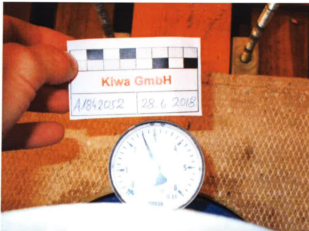
Figure A8. Water tightness test with \geq 2,5 bar water filled test cylinder (manometer after 72 hours on 28.06.2018).
