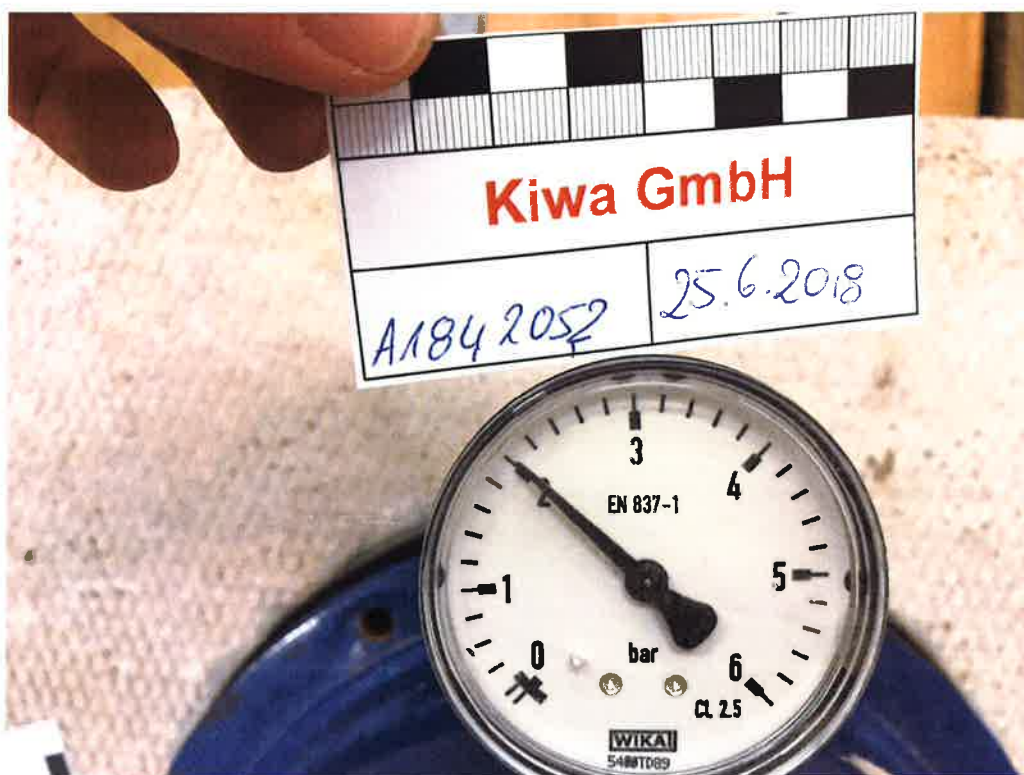
Figure A6. Water tightness test with \geq 2,0 bar water filled test cylinder (manometer after 67 hours on 25.06.2018).
