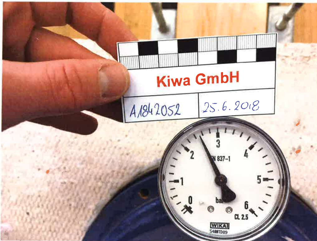
Figure A7. Water tightness test with \geq 2,5 bar water filled test cylinder (manometer at the beginning of testing on 25.06.2018).
