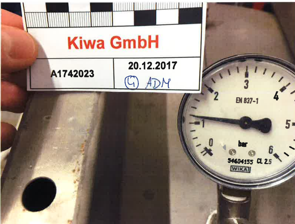
Figure A2. Water tightness test with \geq 1,0 bar water filled test cylinder (manometer after 28 days on 20.12.2017).
