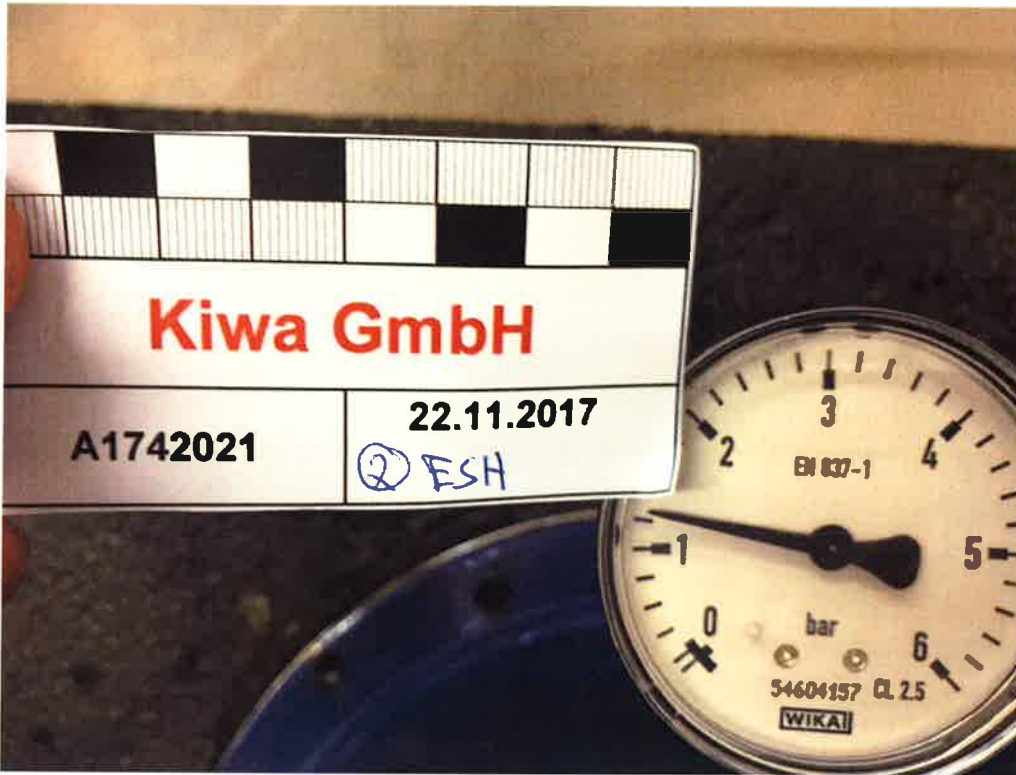
Figure A1. Water tightness test with \geq 1,0 bar water filled test cylinder (manometer at the beginning of testing on 22.11.2017).
