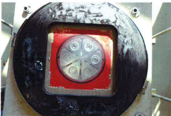
Figure 3. Test block with concrete embedded single wall insert Hauff HSI150-K/150 and system cover Hauff HSI150-DT.
