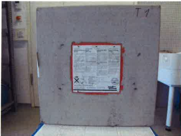
Figure 2. Examples for a test block with embedded single wall insert Hauff HSI150-K/150.
