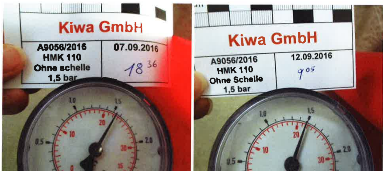
Figure A2. Water tightness test with the 1,5 bar water filled pressure bell (left: manometer on September 7 th , 2016 at 6:36 pm; right: manometer after 4 days on September 12 th , 2016 at 9:05 am).
