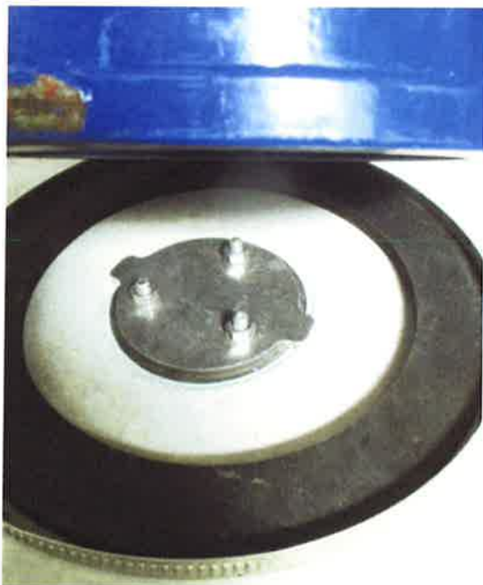
Figure 4. Example for a 40 mm thick EPDM sealing.
