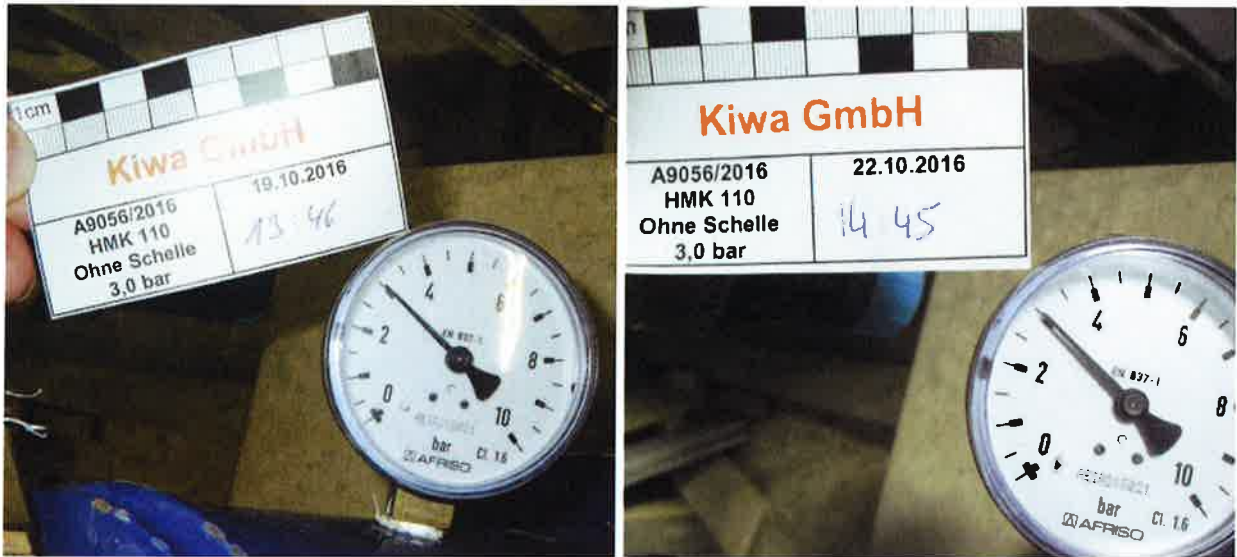
Figure A5. Water tightness test with the 3,0 bar water filled pressure bell (left: manometer on October 19 th , 2016 at 1:46 pm; right: manometer after 3 days on October 22 nd , 2016 at 2:45 pm).
