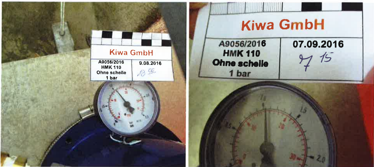
Figure A1. Water tightness test with the 1,0 bar water filled pressure bell (left: manometer at the beginning of testing on August 9 th , 2016 at 6:06 pm; right: manometer after 28 days on September 7 th , 2016 at 7:15 am).
