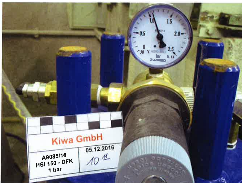
Figure A2. Water tightness test with the \geq 1,0 bar water filled pressure bell (manometer after 28 days on December 5 th , 2016 at 10:11 am).
