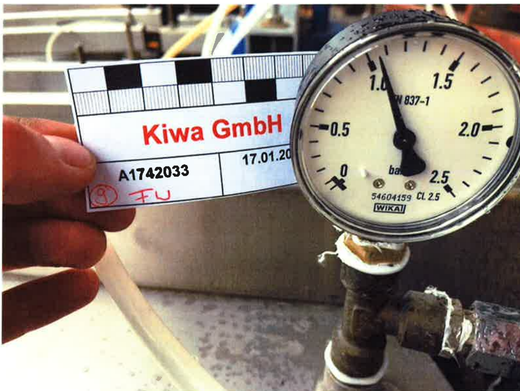
Figure A2. Water tightness test with \geq 1,0 bar water filled test cylinder (manometer after 28 days on 17.01.2018).
