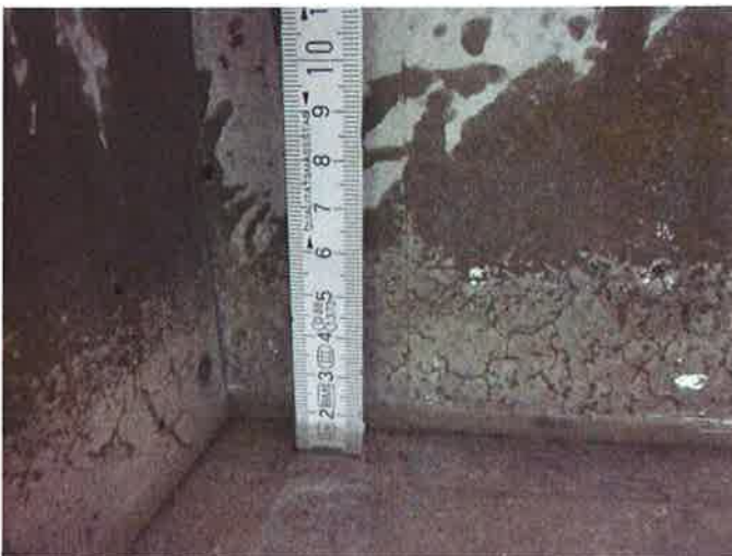
Illustration 14: Oil level in the trough immediately after the insertion of the oil in the area of the pouring location (approx. 16 mm)
