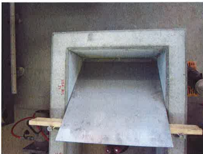
Illustration 10: Sheet steel with base recesses as a pouring help for the insertion of the oil
