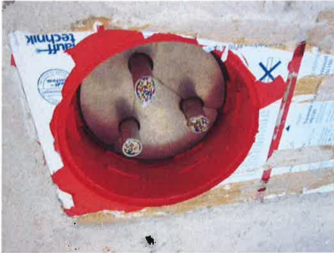
Illustration 21: HSI 150 K2-100 with HRD150/160-G-3/20 (NBR), trough under-side after 92 days
