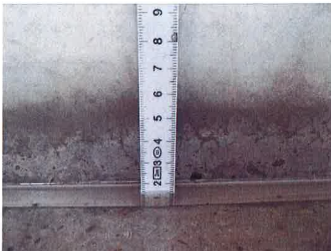
Illustration 16: Oil level in the trough at trial end after 92 days oil impingement contact in the area of the sealing joint (approx. 15 mm)
