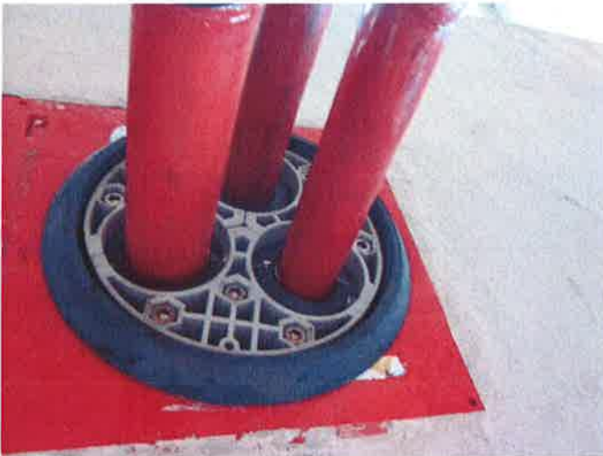
Illustration 18: HSI 150-DG, trough under-side after 92 days
