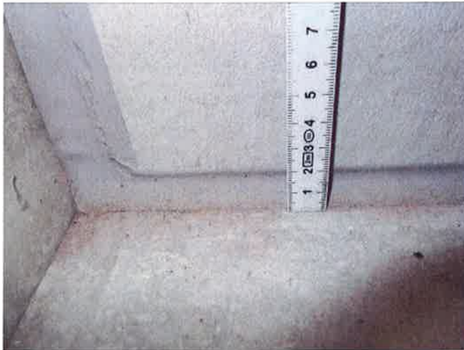
Illustration 25: Sealing joint Sikaflex Tank N on the side facing the oil after 92 days
