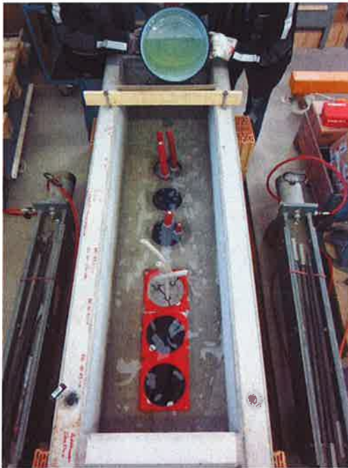
Illustration 12: Pouring the heated oil (90.0°C) into the concrete trough
