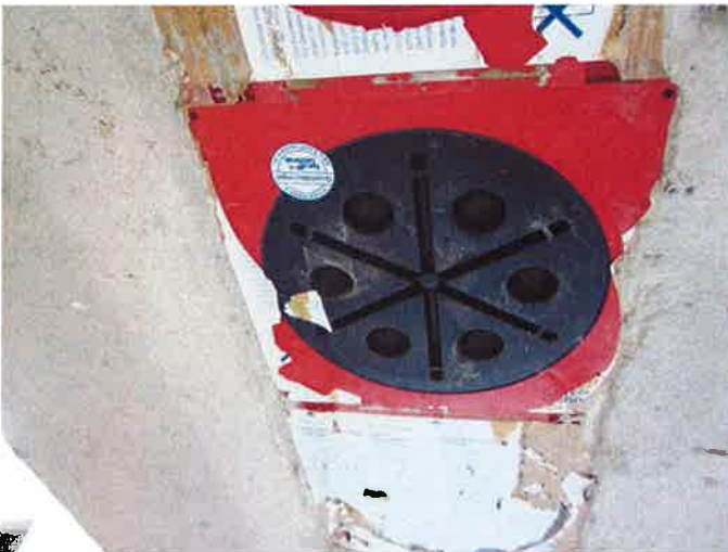
Illustration 22: HSI 150 K2-100 with close-off lid HSI 150-D (1 st experiment), trough under-side after 92 days
