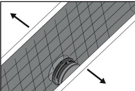
5 After the concrete has hardened, remove the formwork.
