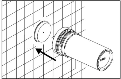
Push the wall sleeve with folding sleeve onto the attached closing cover and position it in the inner formwork.
