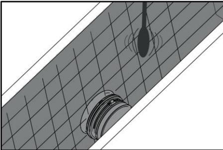
4 Carefully compact the concrete around and between the casing pipe in layers using a vibrator.
