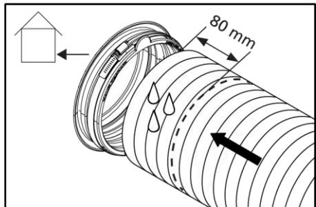
**5** Mark the insertion depth (see Table 1) on the cable protection tube. Push the cable duct into the folding sleeve up to the marking.
