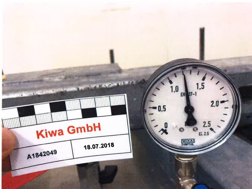
Figure A2. Water tightness test with \geq 1,0 bar water filled test cylinder (manometer after 28 days on 18.07.2018).
