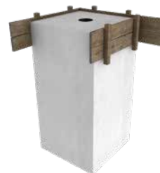
Foundation concreted on-site
