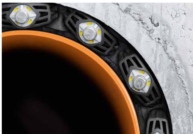
GKD – fully installed, all viewing windows are filled with yellow.
