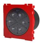
Single wall inserts are available above a wall thickness of 70 mm. In addition to a closing cover, they are also equipped with a safety cover that is not removed until just before the cable is laid.
