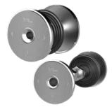
The earthing entry HEA M12 has a specially contoured contact washer for patented twist resistance and is suitable for installation flush with the formwork in waterproof concrete.
