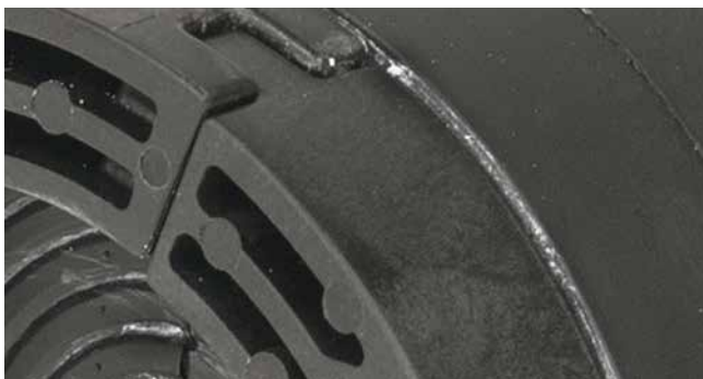
press plate with form-fitting connection
