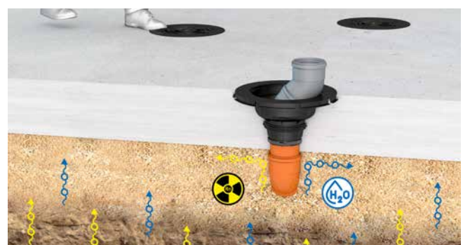
AT110 installed in the floor slab, absolutely gas- and watertight, with the option of tolerance compensation and connection of a vapor barrier
