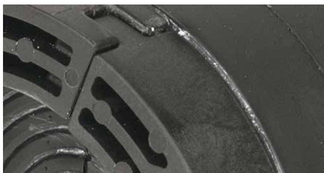
press plate with form-fitting connection
