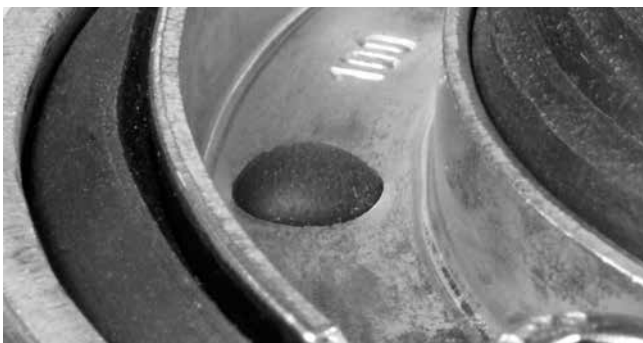
Visual and physical installation control through integrated inspection window
