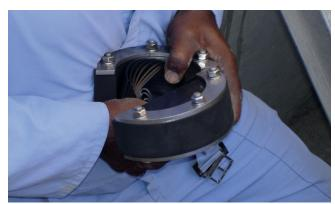
Segmented ring technology the split design allows effortless removal of the individual segmented rings
