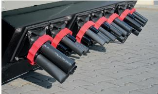
The cloroprene surface sealing fi ts perfectly to the building entry sealings of the station. Thanks to the cathodic dip coating of the aluminium fl anges a optimal corrosion protection was achieved. Sealing of the cables is done by means of heat shrinkable sleeves. Not used openings will be safely closed with a blind plug.
