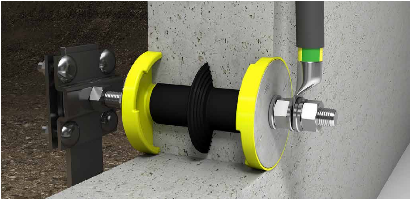
HEA IS M12 earthing entry: a flat steel connection via the KKL M12 cross-clamp on one side and an earthing conductor connection via the ASB M12 connection bolt on the other side.
