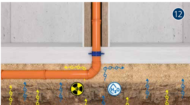
KGF110 set in concrete
