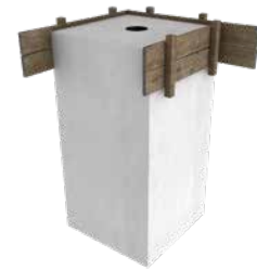
Foundation concreted on-site
