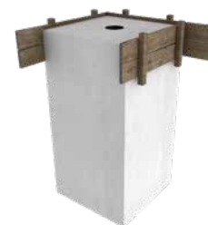
Foundation concreted on-site
