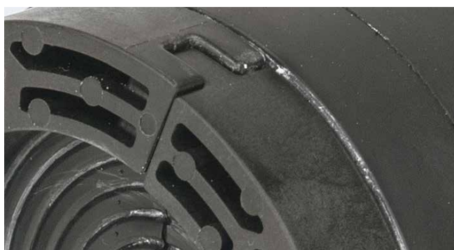
press plate with form-fitting connection
