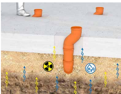
please note: no tight connection between rectangular recess and concrete and between waste water pipe and concrete
