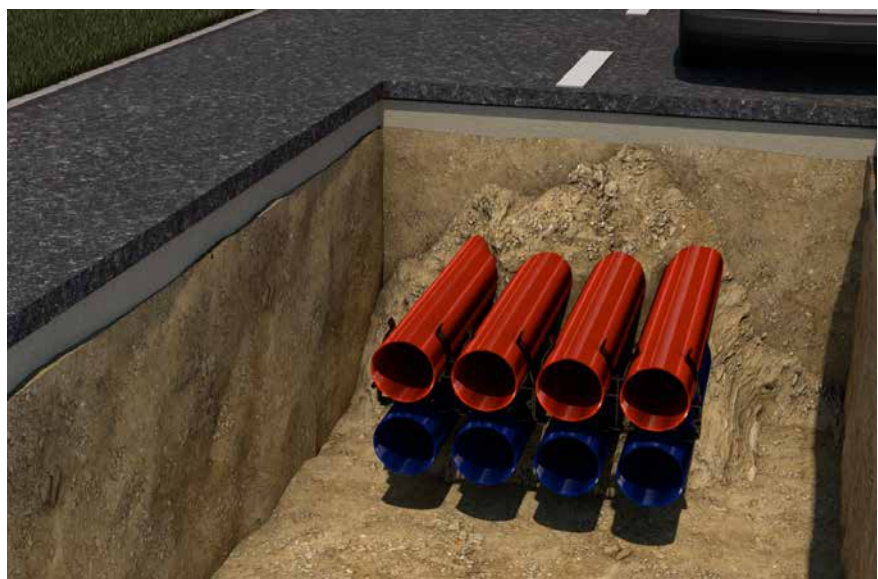
Minimum routing depth of cable ducts for heavy load traffic for heavy trucks
