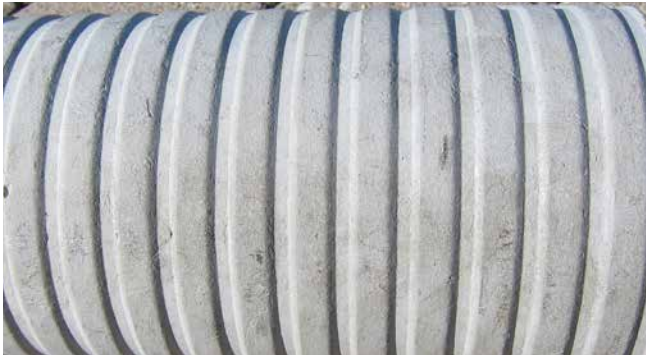
lengthwise watertight outer grooves
